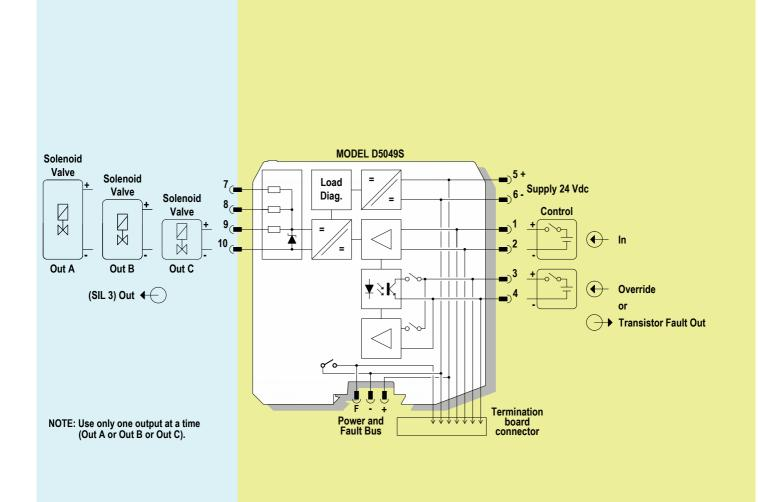
Terminals 3-4 dip-switch selectable for fault output signaling or override control
